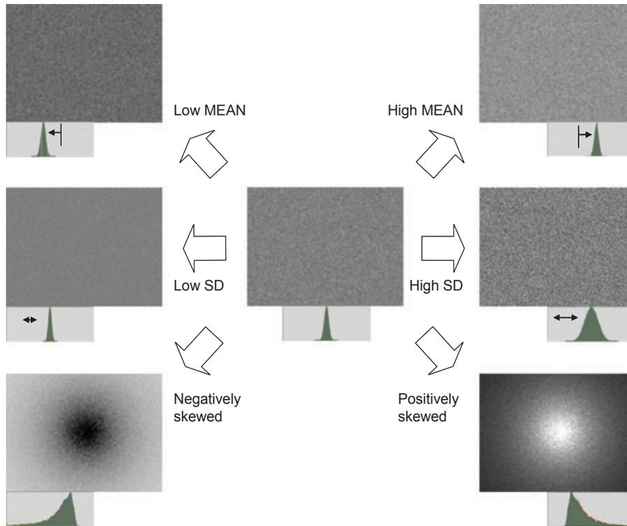
Fig. 3. Concept of the image histogram and the image histogram parameters (mean, standard deviation, skewness) illustrated by synthesized images. The image histogram is a chart showing a distribution of the pixel values in the image. These images are prepared to explain the concept of image histogram analyses by simulating the appearances that appears to the skin. This chart shows how the image histogram parameters are changed when the images look different.
